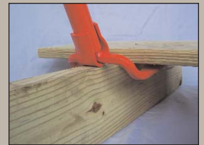
Fits over single floor joist as well as double floor joist.
